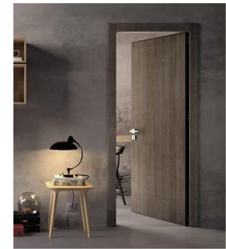
Doors that are flush on the push side open towards the inside of the frame instead of the outside, thanks to the use of concealed hinges. In this way, the leaf and frames can be on the same plane.
