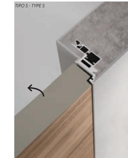
Fire resistant door with extruded aluminum frame to fit in the masonry or in plasterboard 125 mm thick to be sure of EI 60 fire resistance. 60 mm leaf which **can be flush to the wall on pull or push side**. Intumescent gasket on the frame. SOUND INSULATION 28-38-42 db.
